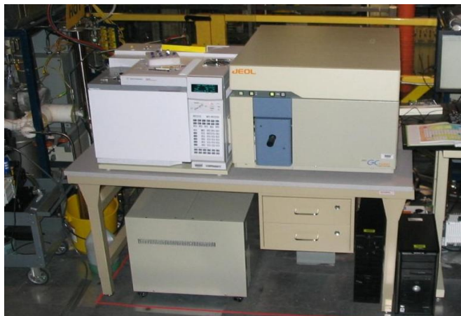
JMS-GCmate II (JEOL Ltd., Japan) high-resolution magnetic sector mass spectrometer installed in TCPDU
